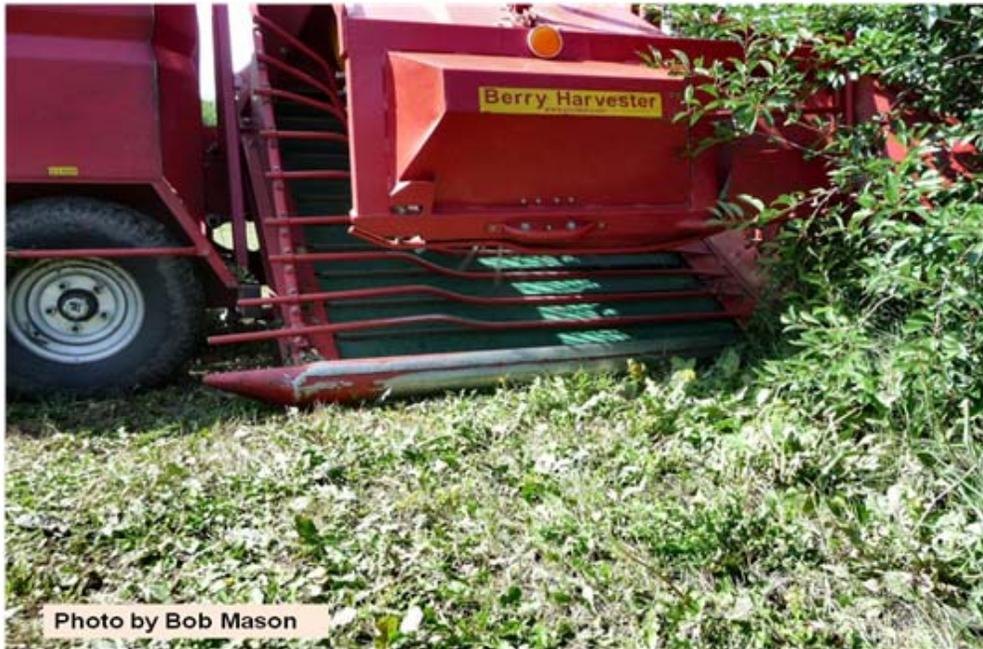
**Figure 2. Joanna Harvester with collector lowered to the ground. It is designed to pick fruit just a few inches off the ground**
